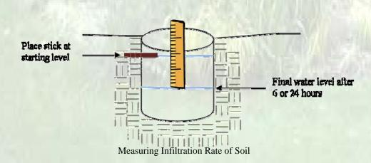
for 24 hours. (Inches of drop in 6 hours x 4= inches of drop in 24 hours) If the level has changed less than one inch after 6 hours, wait a full 24 hours from the time you initially filled the hole and measure the total drop. This measurement will be the amount of water that can soak into the ground in 24 hours (one day). No multiplication is need.
